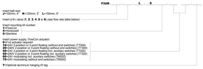
Example: F3UR.J.3.L.S.1.10.T=Unimizer 2-way 100mm (Kv equal to 131 m3/h) with FlowCon mounting kit, 24V 2-position actuator and ID-tag.
